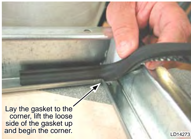
FIG. 5-69 – APPLY GASKET TO CORNER
