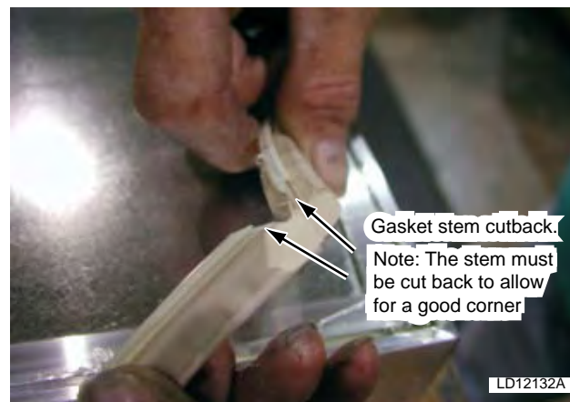
FIG. 5-31 – CUT BACK STEM
