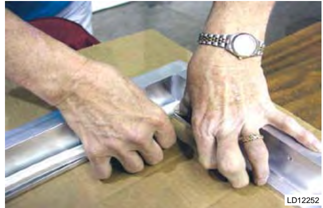
FIG. 5-49 – ATTACH GASKET TO ONE CORNER
