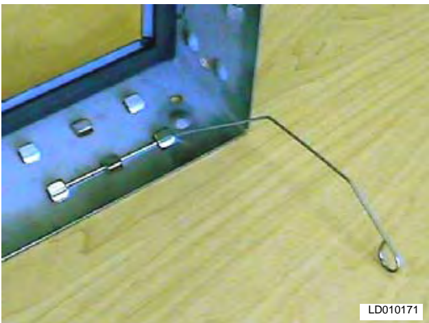
FIG. 2-99 – CORRECTLY INSTALLED LATCH P/N 026-35778-000.
