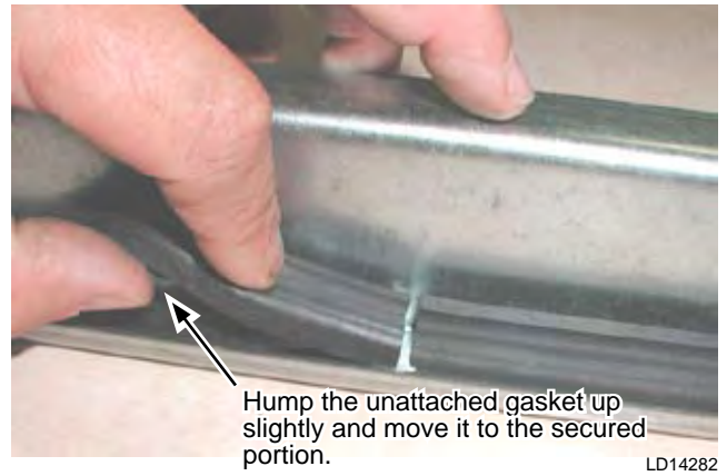
FIG. 5-78 – POSITION GASKET FOR SECURING
