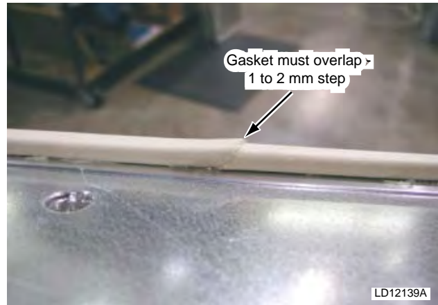
FIG. 5-38 – OVERLAP CUT PIECE WITH “IN PLACE” GASKET
