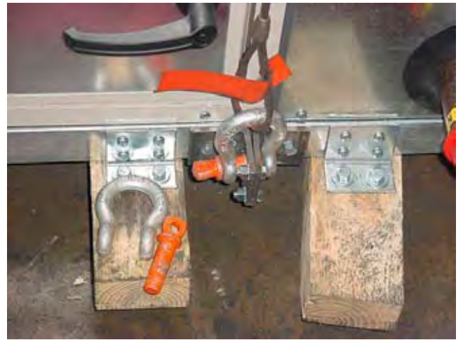
FIG. 1-5 – PROPER LIFTING WITH SHACKLE AT LIFTING LUG
