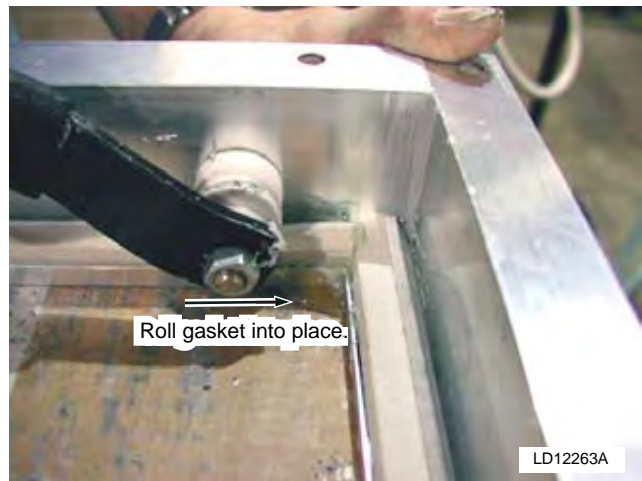
FIG. 5-60 – ROLL VERTICAL GASKET INTO PLACE AND SECURE
