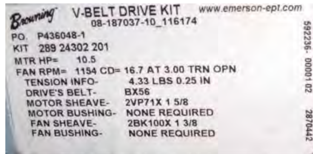
FIG. 4-2 – TYPICAL DRIVE KIT DATA TAG
