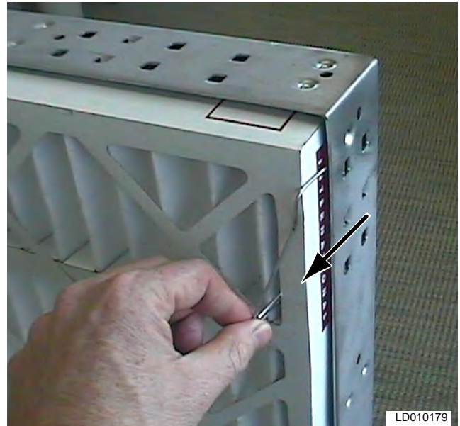
FIG. 4-24 – PLACE THE END OF THE LATCH OVER THE FILTER FRAME, SECURING THE FILTER TO THE FRAME.
