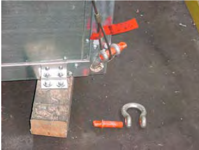
FIG. 1-4 – PROPER LIFTING WITH SHACKLE AT CORNER
