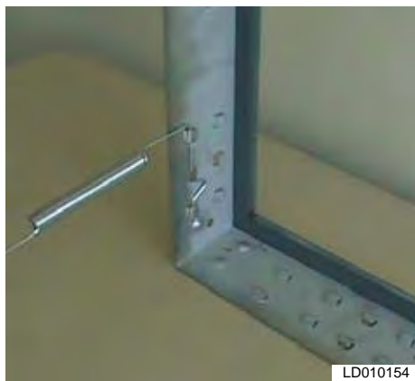
FIG. 2-107 – CORRECT LATCH/KNOCKOUT CONFIGURATION.
