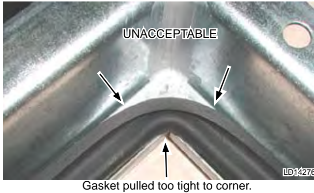
FIG. 5-72 – UNACCEPTABLE CORNER - TOO TIGHT
