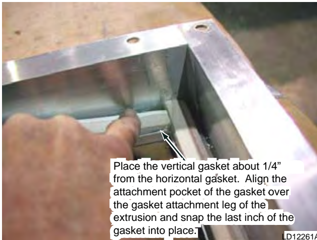
FIG. 5-58 – POSITION VERTICAL GASKET
