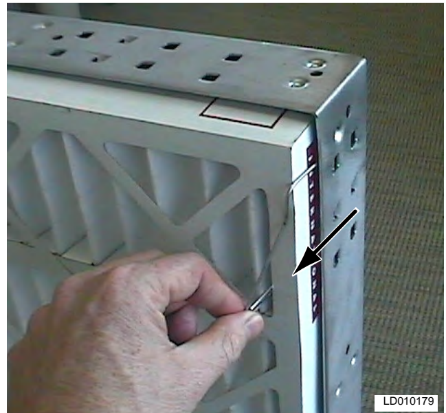
FIG. 2-102 – PLACE THE END OF THE LATCH OVER THE FILTER FRAME, SECURING THE FILTER TO THE FRAME.
