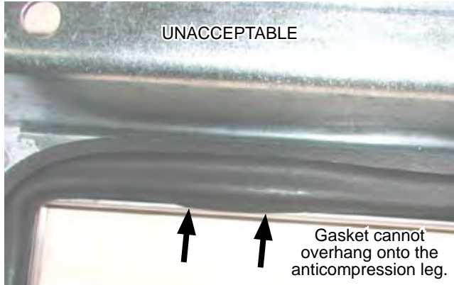
FIG. 5-76 – UNACCEPTABLE GASKET FIT - GASKET OVERHANGS ANTICOMPRESSION LEG.
