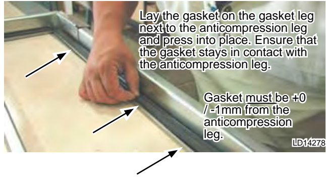
FIG. 5-74 – LAY GASKET ON GASKET LEG
