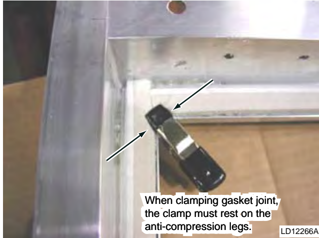
FIG. 5-63 – APPLY CLAMP TO CORNER AS NECESSARY
