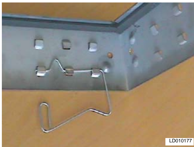
FIG. 4-23 – CORRECTLY INSTALLED LATCH P/N 315-004-000
