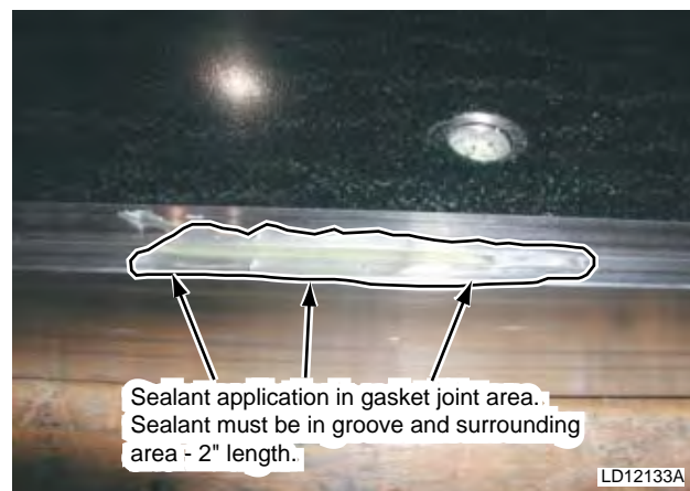
FIG. 5-32 – APPLY SEALANT TO OVERLAPPING SPLICE AREA
