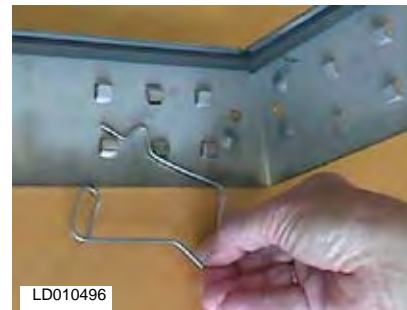
FIG. 2-104 – INSTALL LATCH P//N 026-35778-007
