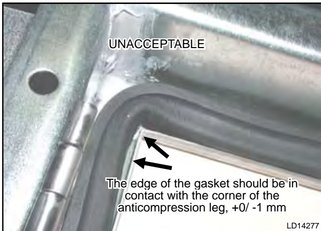
FIG. 5-73 – UNACCEPTABLE CORNER - GASKET EDGE NOT TOUCHING CORNER OF ANTICOMPRESSION LEG.
