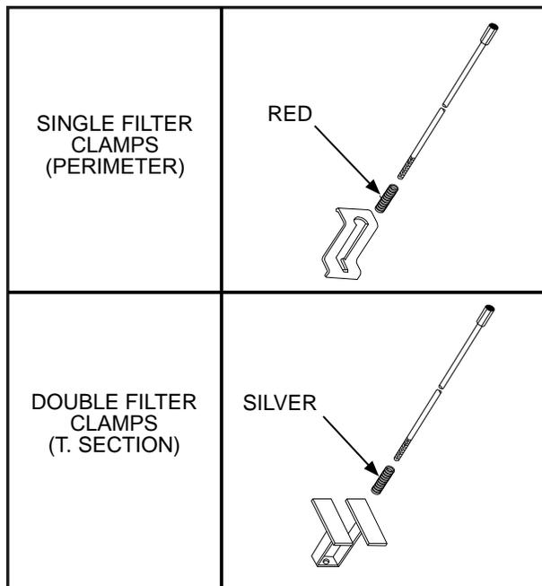
Used to attach HEPA Filters to Holding Frame.
