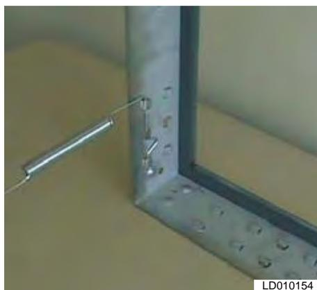
FIG. 2-107 – CORRECT LATCH/KNOCKOUT CONFIGURATION.
