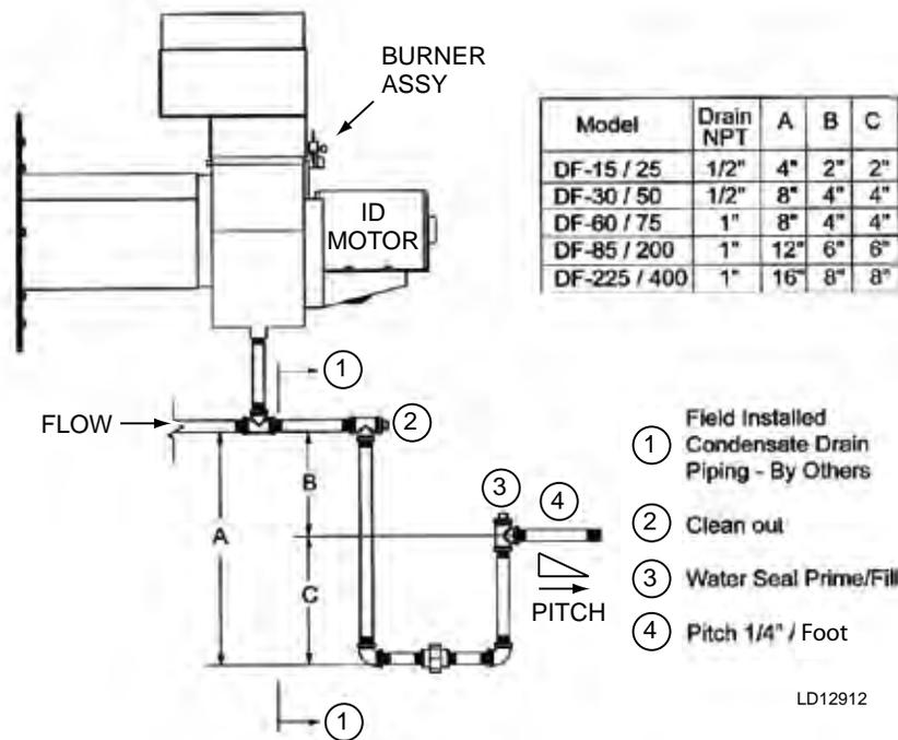
FIG. 2-53 – GAS FURNACE CONDENSATE DRAIN TRAP
