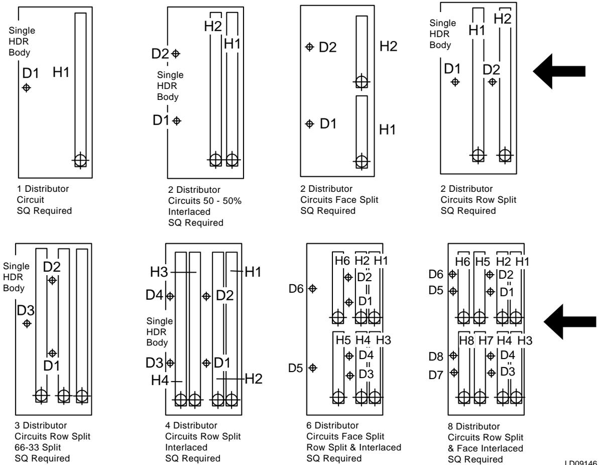
FIG. 2-82 – STACKED COIL DESIGNS - SQ SPECIAL
