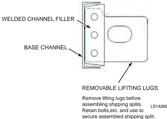
**FIG. 2-26 – REMOVE LIFTING LUGS AND SAVE HARDWARE**
