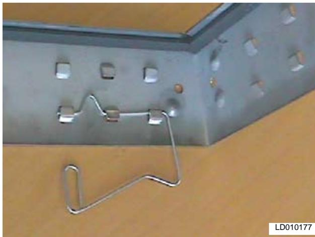
**FIG. 2-101 – CORRECTLY INSTALLED LATCH P/N 026-35778-007**
