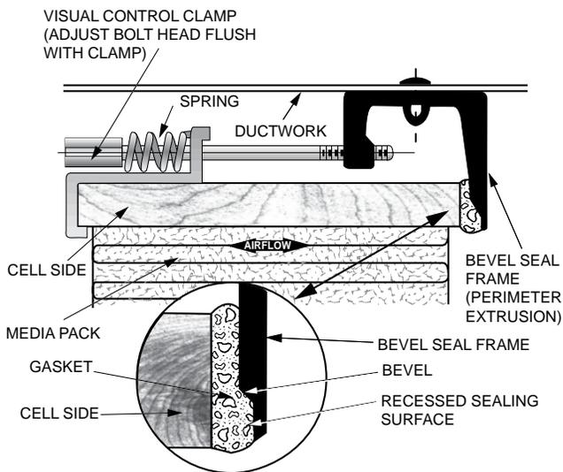
**FIG. 2-119 – WELDED BEVEL SEAL FILTER INSTALLATION**
