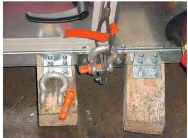
**FIG. 1-5 – PROPER LIFTING WITH SHACKLE AT LIFTING LUG**
