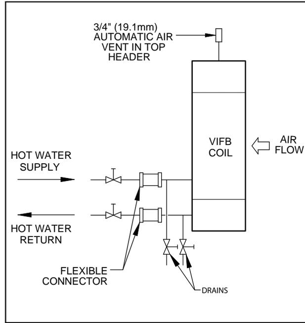
FIG. 2-74 – HOT WATER PIPING FOR 2 ROW COIL VIFB
