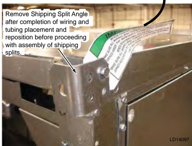
**FIG. 2-19 – REMOVE AND REPOSITION SHIPPING SPLIT ANGLE**
