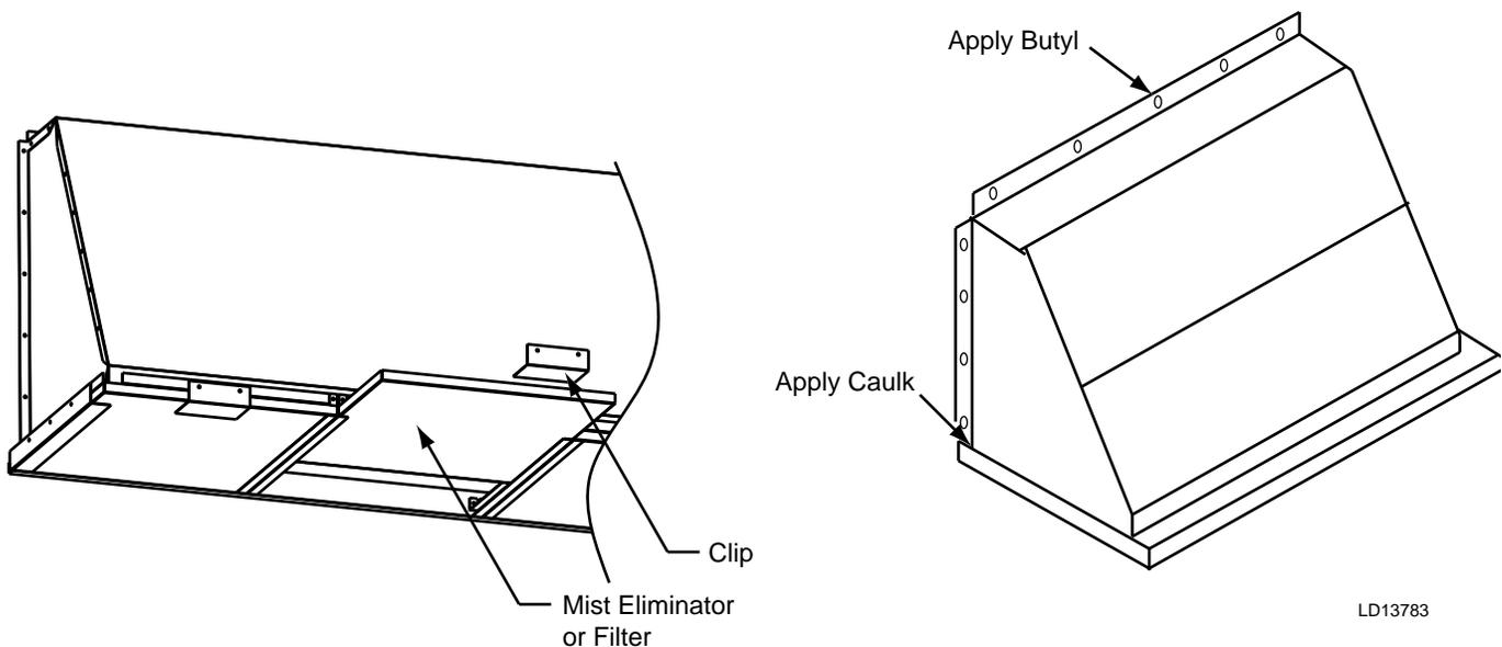
FIG. 2-34 – HOOD INSTALLATION WITH OPTIONAL MIST ELIMINATORS
