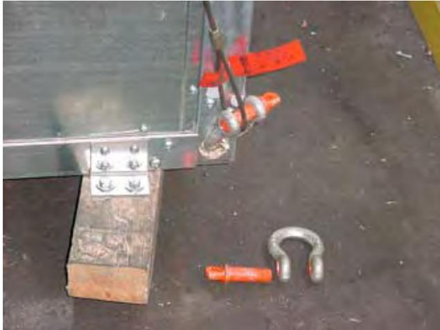
**FIG. 1-4 – PROPER LIFTING WITH SHACKLE AT CORNER**
