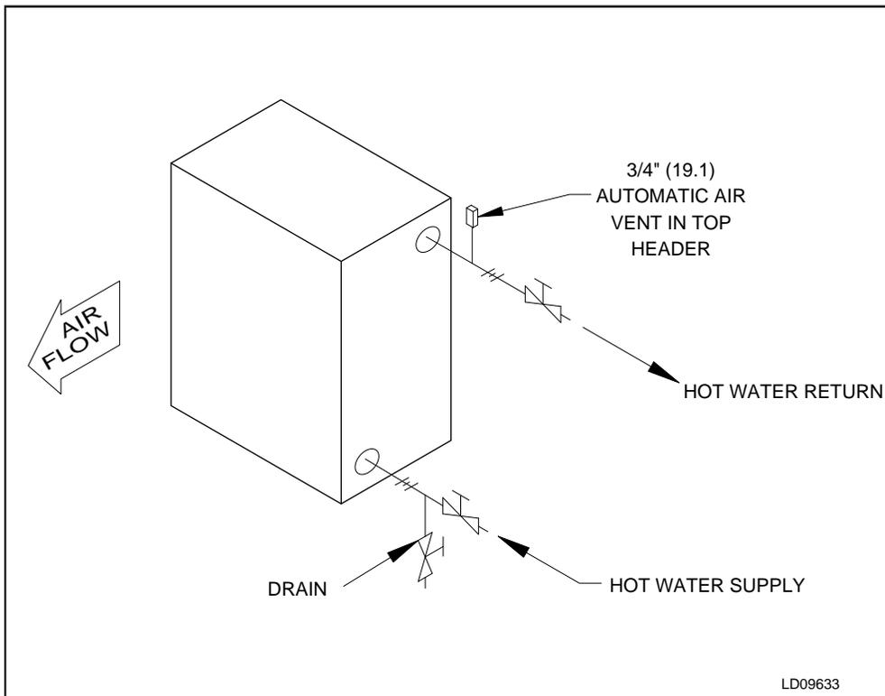
FIG. 2-75 – HOT WATER PIPING FOR IFB
