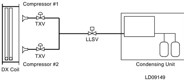
**FIG. 2-85 – TWO COIL CIRCUITS PER REFRIGERANT CIRCUIT**
