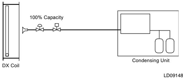
**FIG. 2-84 – ONE COIL CIRCUIT PER REFRIGERANT CIRCUIT**
