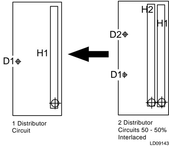
FIG. 2-80 – NON-STACKED COIL DESIGN - STANDARD
