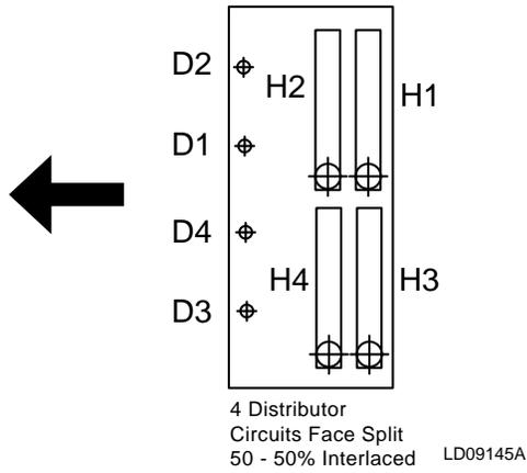
FIG. 2-81 – STACKED COIL DESIGN - STANDARD
