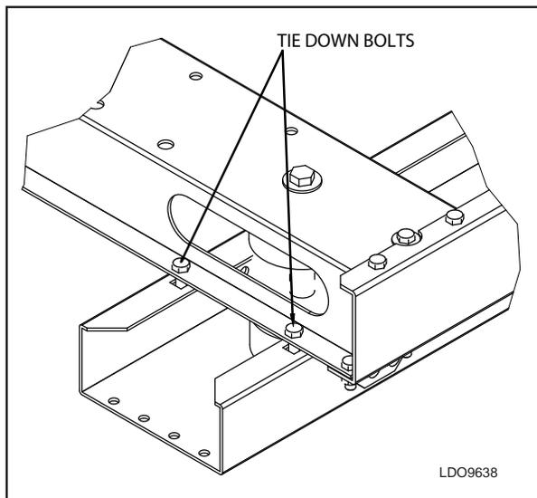
**FIG. 3-2 – FAN AND MOTOR ISOLATOR SUPPORT FRAME.**
