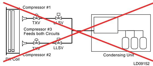
**FIG. 2-88 – DO NOT USE THE ABOVE CONFIGURATION.**
