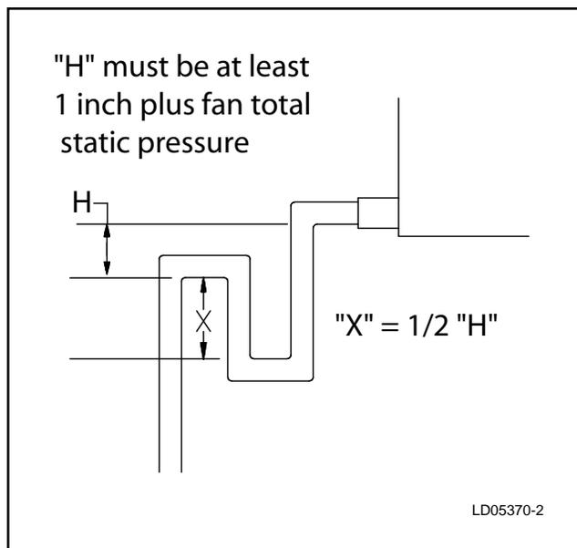
**FIG. 2-91 – TRAP DETAIL FOR DRAW THROUGH APPLICATION**
