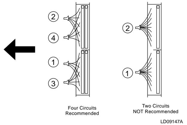
FIG. 2-83 – STACKED COIL CIRCUITING
