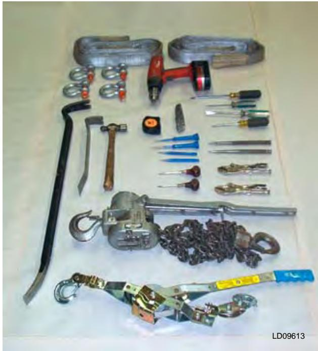
**FIG. 2-7 – TOOLS TYPICALLY USED FOR ASSEMBLY OF SHIPPING SPLITS**
