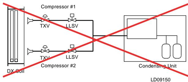
**FIG. 2-86 – DO NOT USE THE ABOVE CONFIGURATION.**
