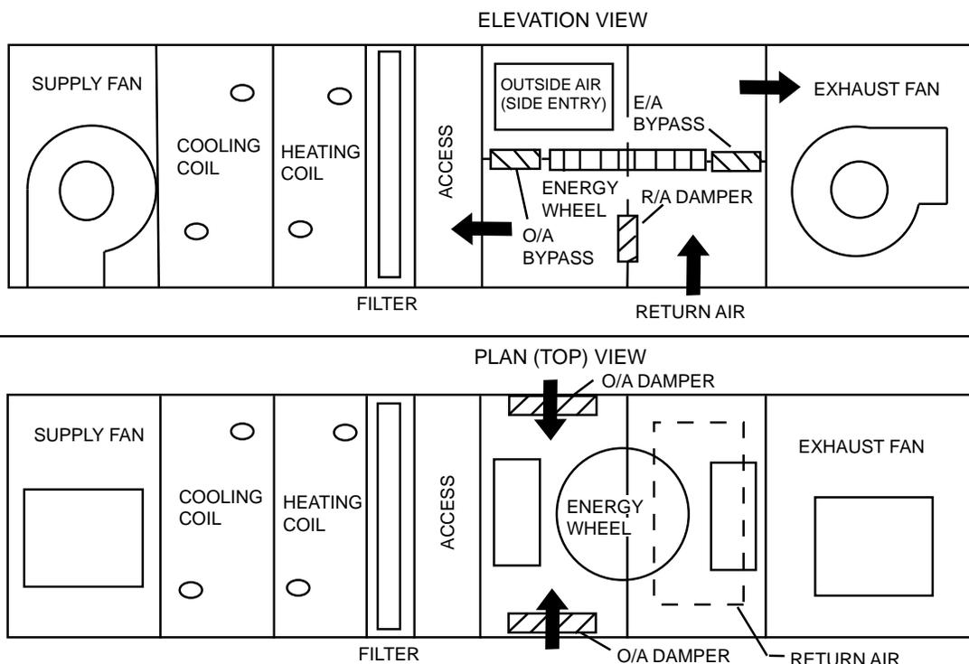
**FIG. 3-10 – OUTDOOR UNIT - HORIZONTAL WHEEL**
