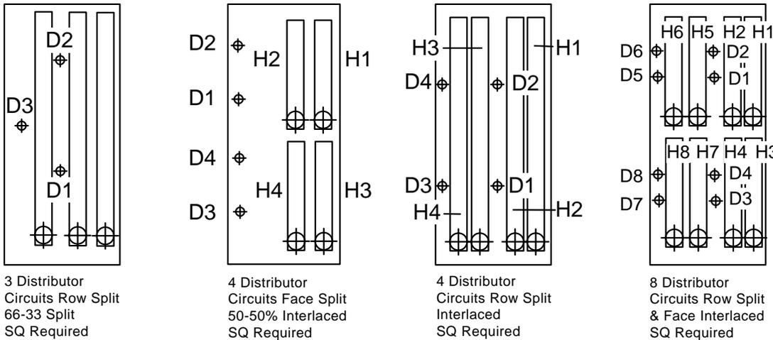
FIG. 2-79 – NON-STACKED COIL DESIGN - SQ SPECIAL
