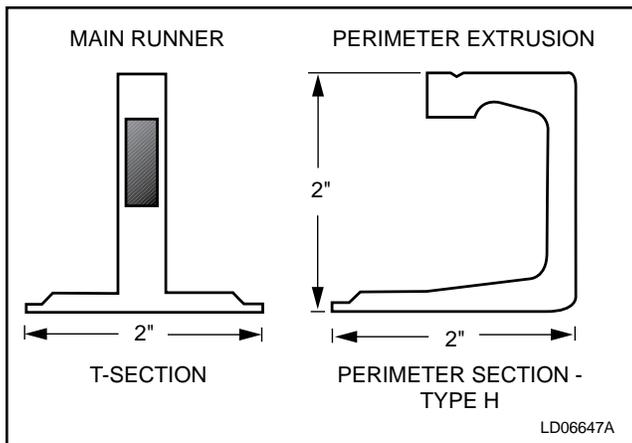
**FIG. 2-116 – HEPA FILTER FRAME CROSS SECTION VIEW**
