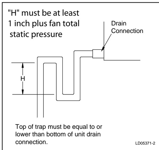
**FIG. 2-92 – TRAP DETAIL FOR BLOW THROUGH APPLICATION**
