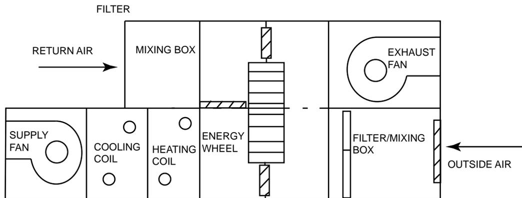
**FIG. 3-9 – INDOOR UNIT - VERTICAL WHEEL**
